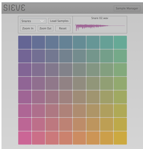
Figure 1: Sieve Plugin UI . Sample type is selected using the drop-down menu and "load samples" button. Samples are auditioned by clicking on the pads of the 2D grid. Areas of the grid can be further explored using the "zoom in" button.
